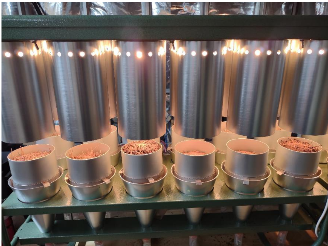
Figure 2.1: Tullgren funnel set-up
